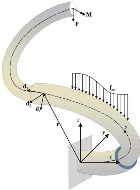
Figure 12. Soft robotic manipulator modelled by using the Cosserat rod approach, with the backbone position ( $\mathbf{r}$ ) and orientation ( $\mathbf{d}_1$ ,  $\mathbf{d}_2$ ,  $\mathbf{d}_3$ ) parametrised by a single variable  $s$ . The manipulator is acted upon by distributed force ( $\mathbf{f}$ ) and discrete forces ( $\mathbf{F}$ ) and moments ( $\mathbf{M}$ ).
